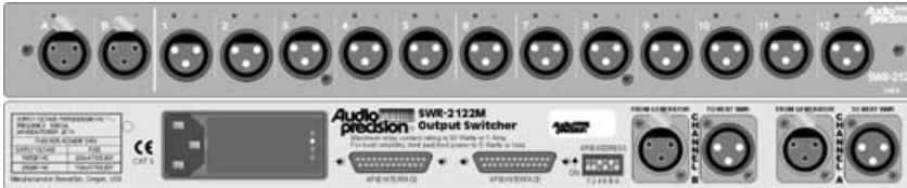
Figure 272. An Audio Precision SWR-2122M Output Switcher, front and rear panels.
